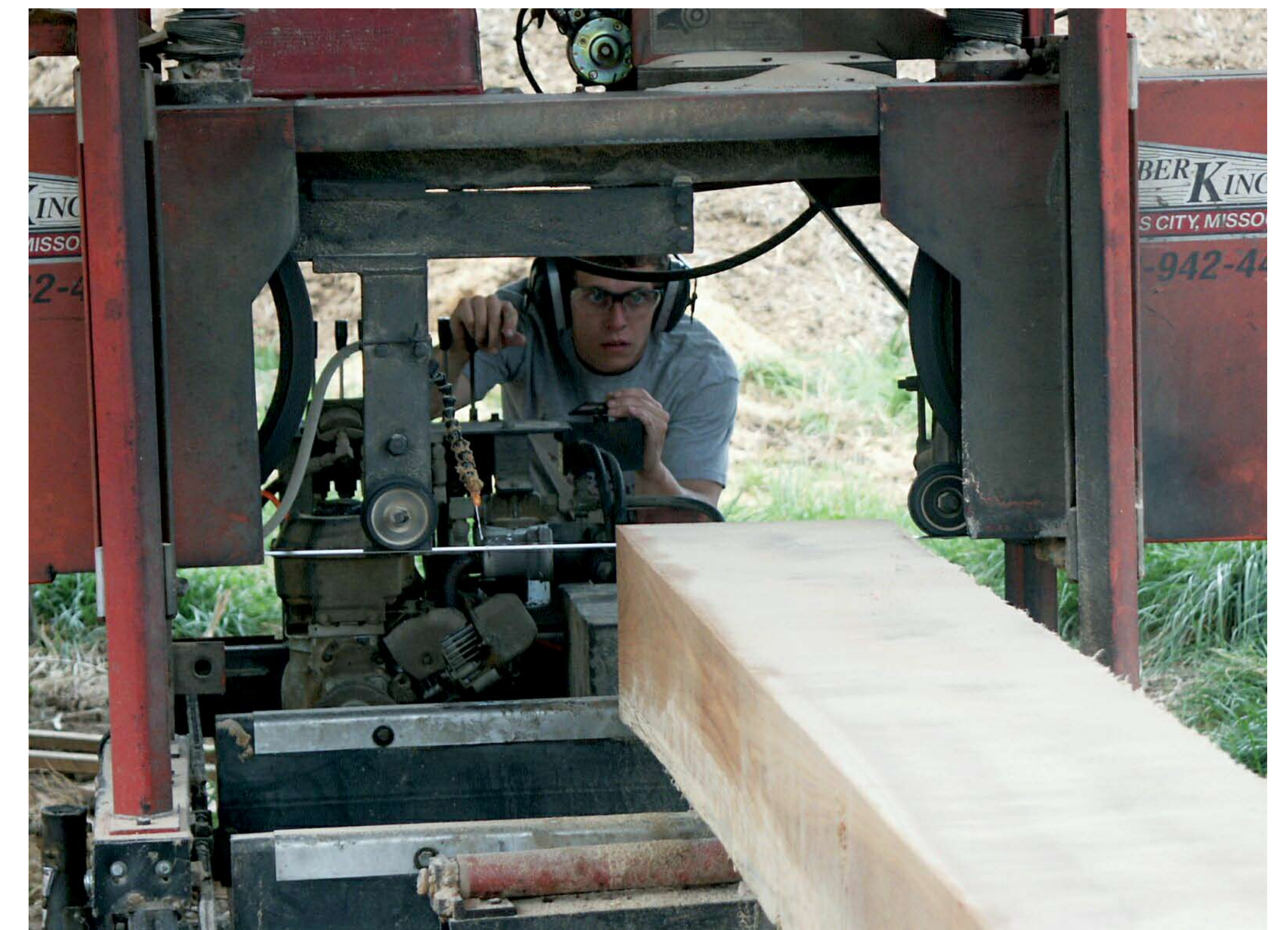
The Forestry Crew operates a College-owned sawmill for preparing timber harvested from its forests. The sawmill produces thousands of board feet of lumber each year for campus projects and public sale.
