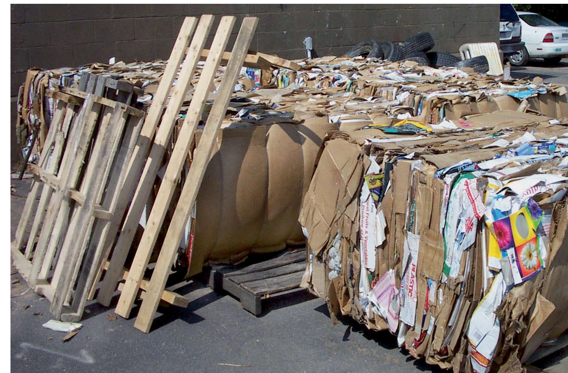
Baling cardboard at the Recycling Center creates income and reduces off-site hauling.
